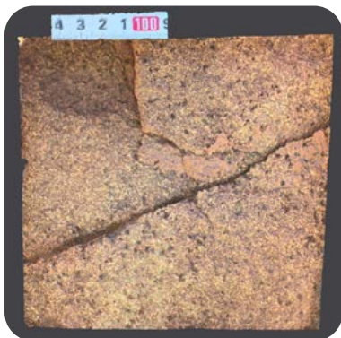
A 2D extract of a typical smartphone imaged 3D model. The dimensions of the rock surface are approximately 100mm x 100mm
